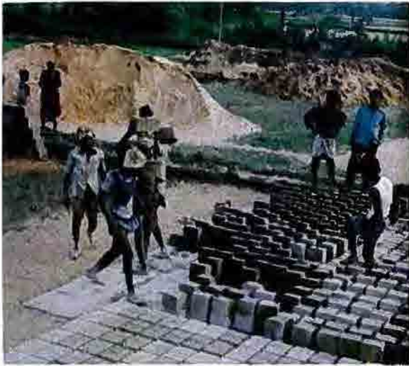
Rural housing using indigenous building material and technology—casting of blocks
